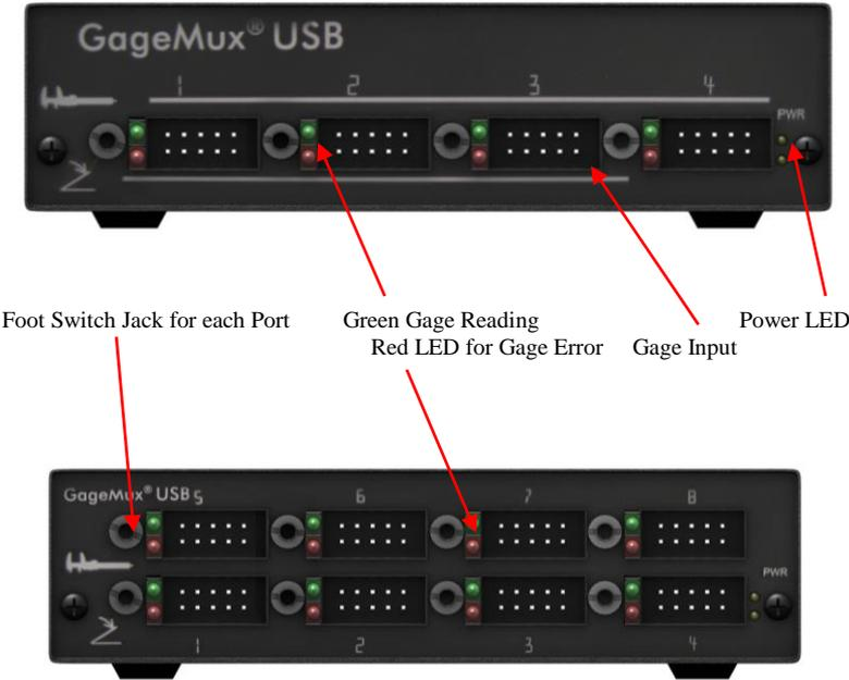
**Figure 1; GageMux® 4 & 8 Port USB Front Panel**
