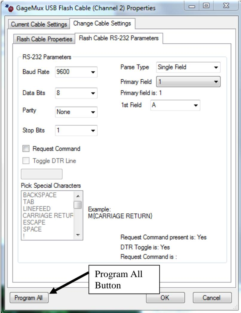
16. Choose Baud Rate, Data Bits, Parity, Stop Bits, by choosing the appropriate setting from the drop down.
